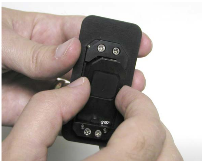
Figure 4.10. Removing a slit from an input adapter.
