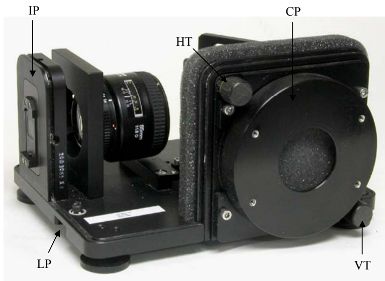
Figure 2.4. Interior of the HoloSpec f/1.4-2.2 , showing the latch pocket (LP), input adapter support plate (IP), camera mounting support plate (CP), horizontal tilt adjustment screw (HT), and vertical tilt adjustment screw (VT).
