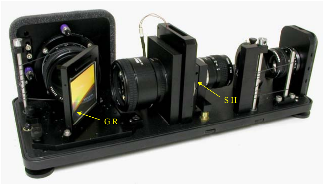
Figure 2.1. Interior of the HoloSpec f1.8i , showing the VPH grating and mount (GR) and the internal slit holder assembly (SH).
