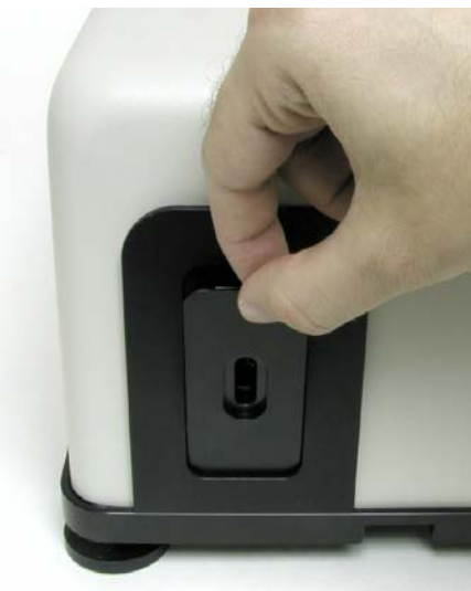
Figure 4.7. Installing the input adapter.
