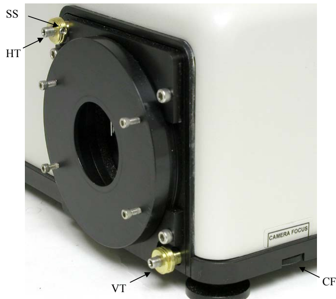
Figure 4.9. The camera mount, including the horizontal tilt knob (HT) with its setscrew (SS), vertical tilt knob (VT), and camera focus thumbwheel (CF).
