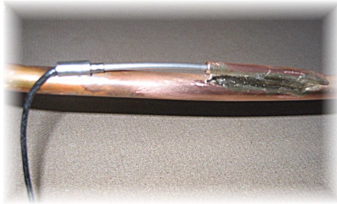
Diagram 15 Remote sensor attached to copper line.
