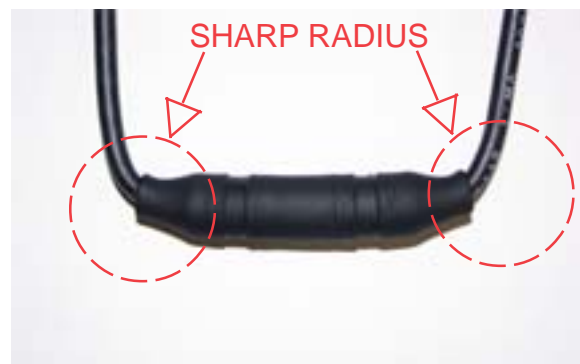
INCORRECT Routing of Cable
